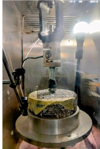
Figure 2. Photo of the indentation test setup.
