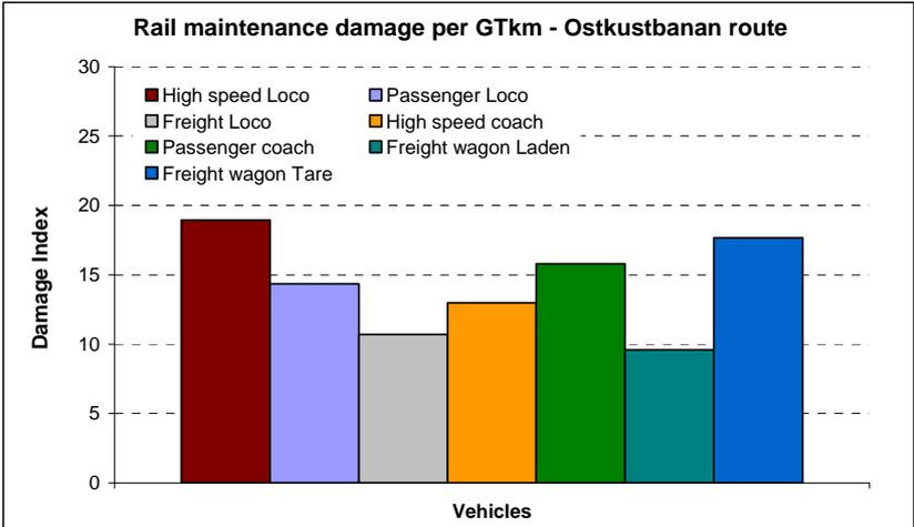
Figure: 9 Rail damage per GTkm by vehicle
