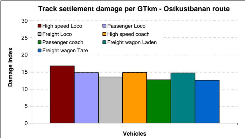
Figure: 8 Track settlement damage per GTkm by vehicle
