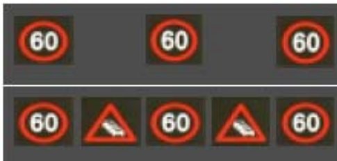
Figure 3.1 Examples of signs displayed above a three-lane-road outside Munich. The upper signs have a shorter perception time than the lower signs. Steinhoff et al., 2000.
