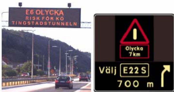
Figure 3.3 Left: Sign showing “E6 Accident, Risk of queue, Tingstad tunnel”. Right: Sign showing “Accident 7 km, Choose E22 S, 700 m”. Kronborg, 2001.
