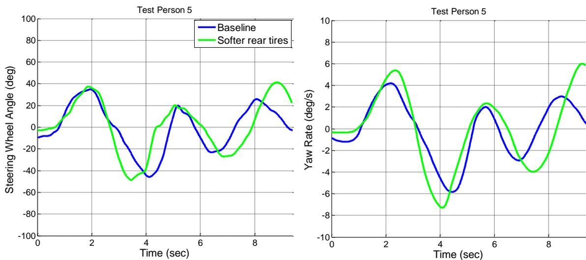
Figure 13. Driver input (steering wheel angle) and truck yaw rate during lane change with baseline truck vs. truck with softer rear tires.
