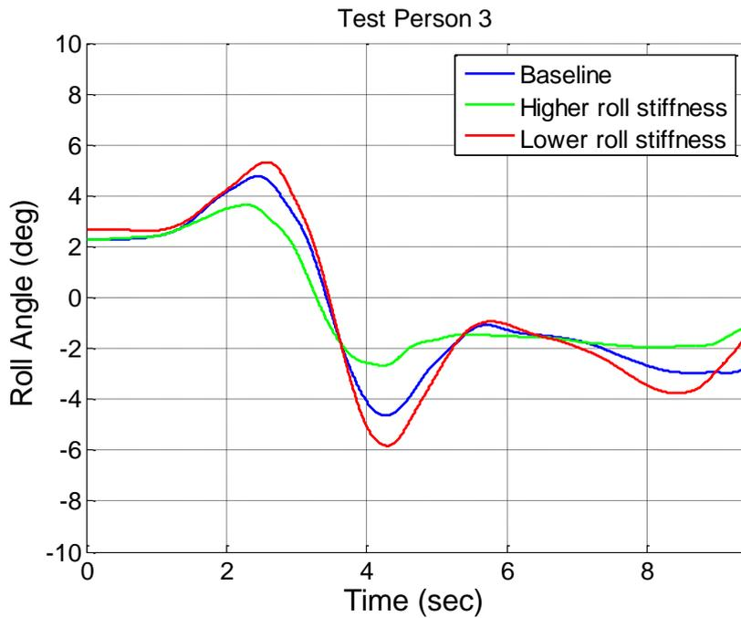
Figure 10. Cabin roll angle during lane changes with trucks with different roll stiffness.
