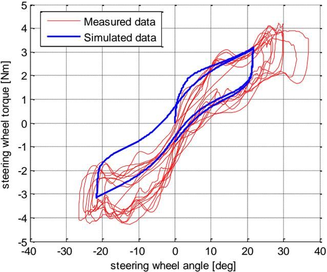
Figure 4. Steering torque of the truck model versus measurements, at 90 km/h.
