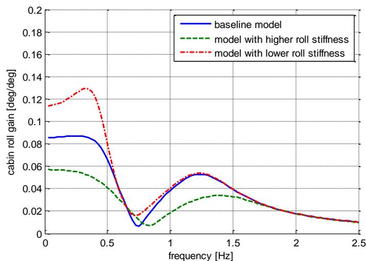
Figure 5. Cabin roll of the baseline model in comparison with a model with parameter sets 1 (higher roll stiffness) and 2 (lower roll stiffness), at 70 km/h.
