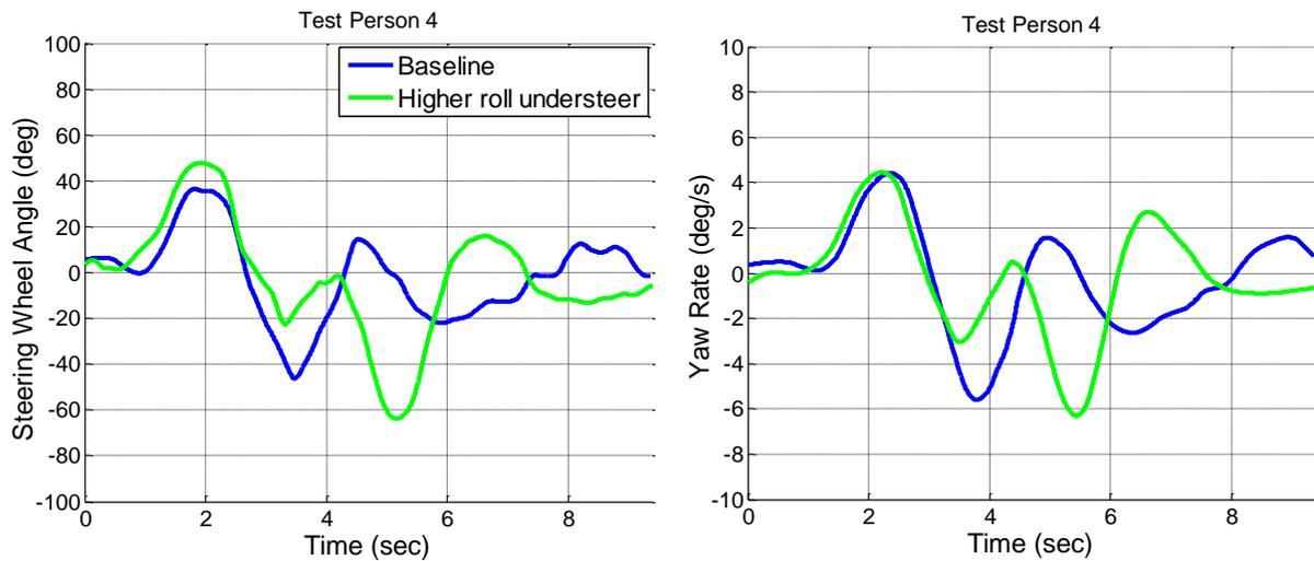
Figure 12. Driver input (steering wheel angle) and truck yaw rate during lane change with baseline truck vs. truck with higher roll understeer.
