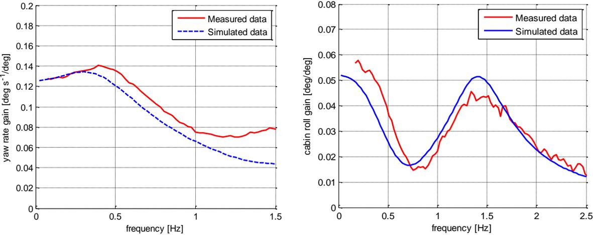
Figure 3. Yaw rate and cabin roll gains with respect to steering wheel angle at 90 km/h. Model outputs versus measurements.
