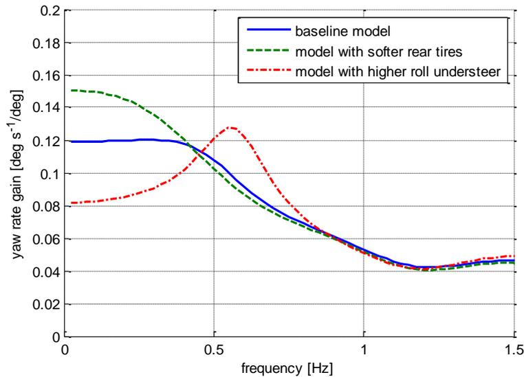
Figure 7. Yaw rate gain of the baseline model in comparison with a model with parameter sets 3 (softer rear tires) and 4 (higher roll understeer), at 70 km/h.
