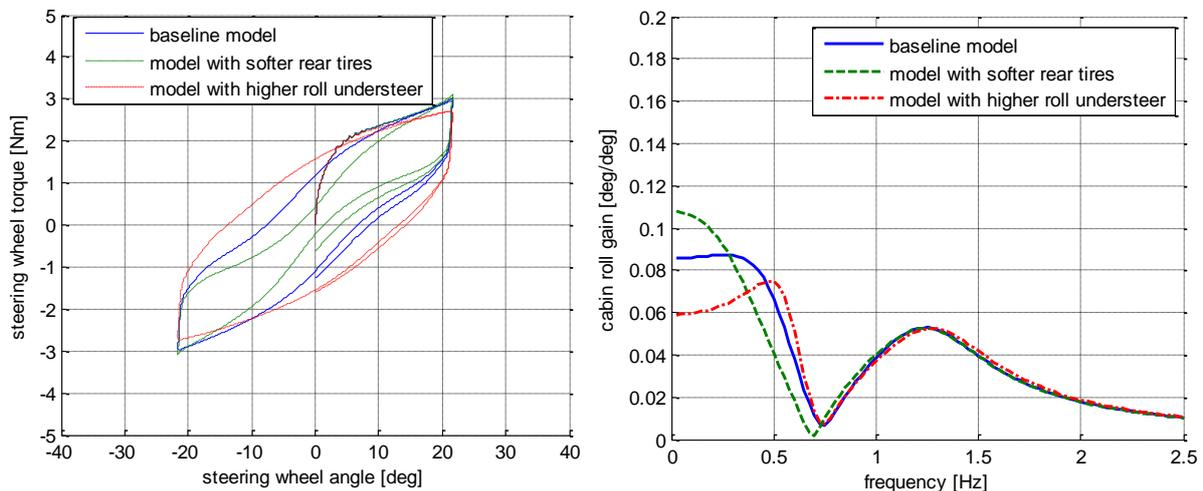
Figure 8. Effects of soft rear tires (parameter set 3) and roll understeer (parameter set 4) on steering wheel torque and cabin roll gain, at 70 km/h.
