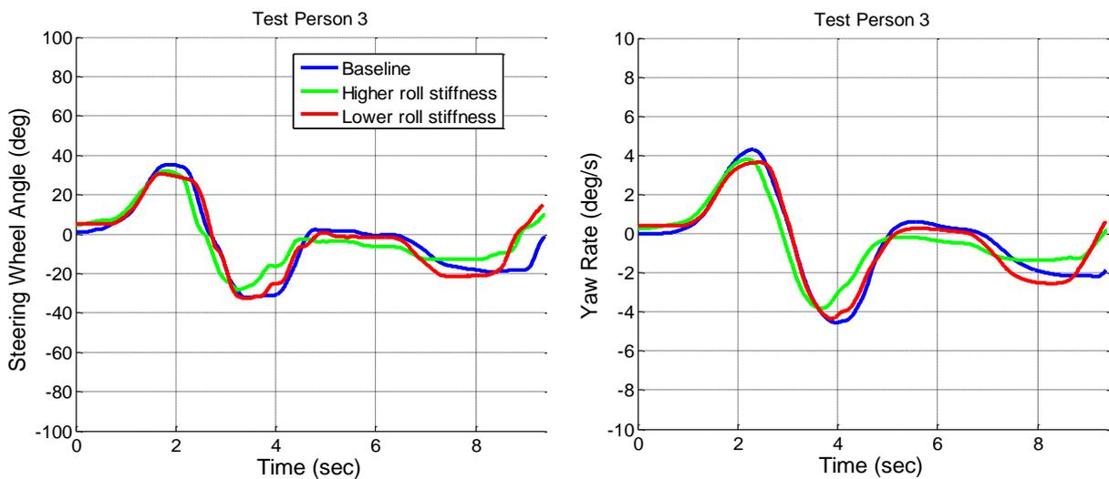
Figure 11. Driver input (steering wheel angle) and truck yaw rate during lane changes with trucks with different roll stiffness.
