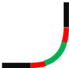
*Figure 9. Curved geometry pattern. In black are the straight sections, in red the transition curves (clothoids) and in green the arc.*
