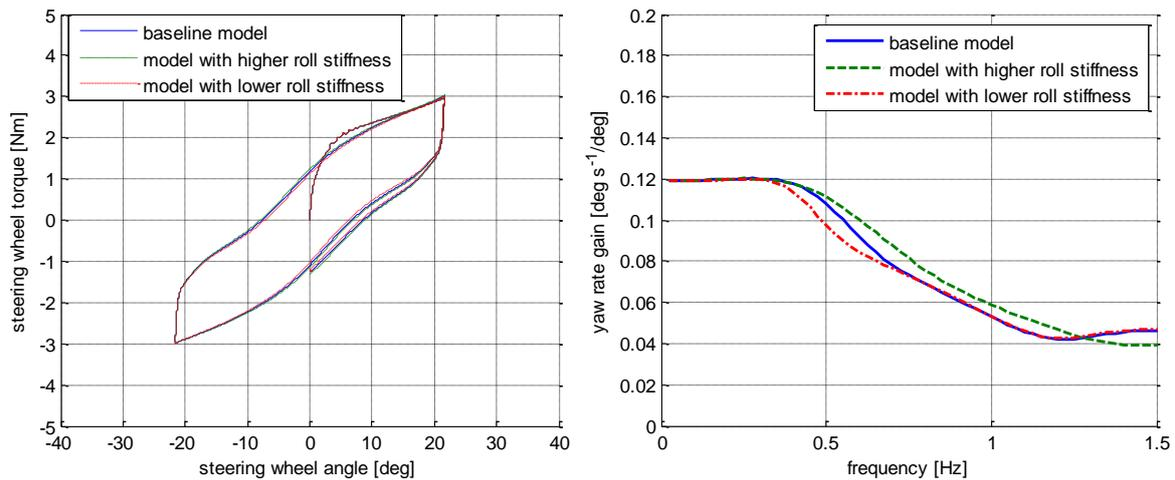
Figure 6. Effects of roll stiffness changes on steering wheel torque and yaw rate gain. Baseline model in comparison with a model with parameter sets 1 (higher roll stiffness) and 2 (lower roll stiffness), at 70 km/h.
